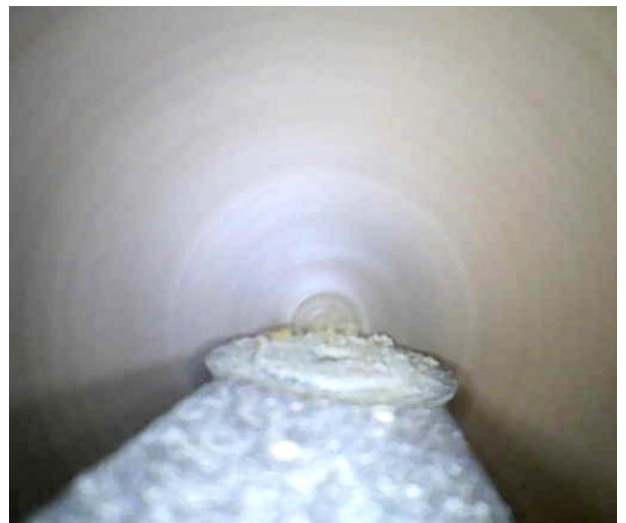
Cutter just approaching nub at inside bottom ↑
