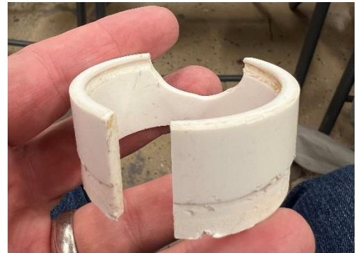
PVC jig Tom Deneen made to hold his small scoops in a 4 jaw chuck for hollowing
