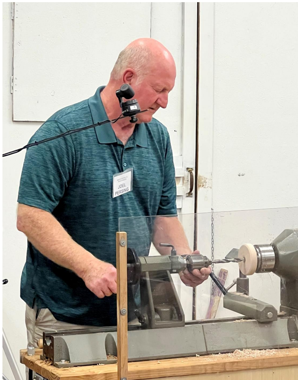
President Joel bores a hole in blank during his demonstration on vacuum chucks at the September meeting
