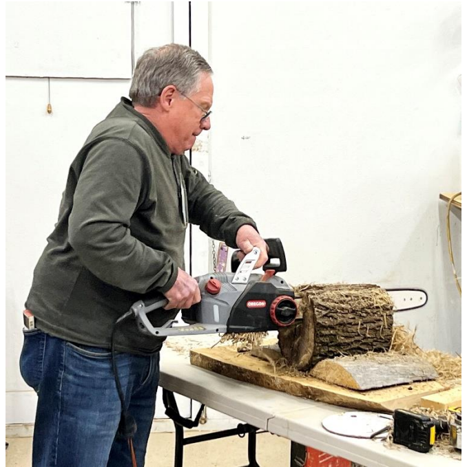
Rich Conley demonstrating preparation of bowl blanks using a chainsaw
