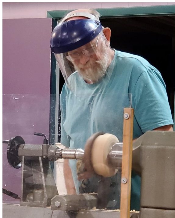
Tom Deneen using a jam chuck in his demo
