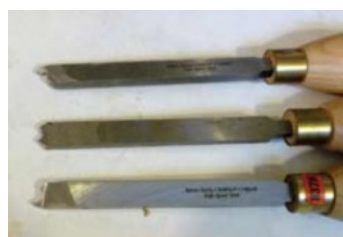
Figure 7. The Robert Sorby tools used in this project: (top to bottom) Right hand side tool, beading tool, and left hand side tool.
