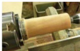
Figure 1. Here the wood has been turned round and to about 1-1/2" in diameter.
