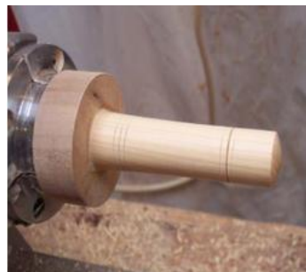
In this photo, the outside of the needle case has been turned and it is ready to part off just in front of the disk holding it in the chuck.
