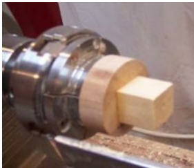
The lid is ready to drill with a 7/16" drill to a depth of about 1/2".
