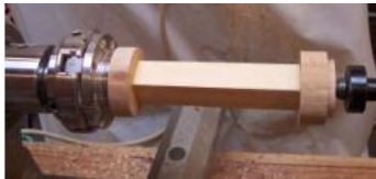
The blank with two disks glued to the ends for greater stability when threading.
