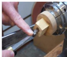
The lid is ready to drill with a 7/16" drill to a depth of about 1/2".
