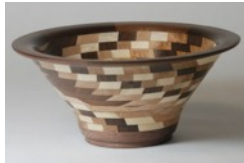
Segmented bowl made of walnut, birch and oak pieces cut with a band saw.
