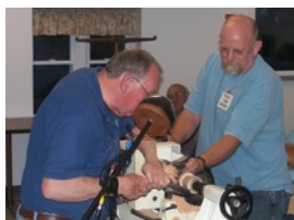
Tom acts as a steady rest to hold the stem as Don finishes the goblet.
