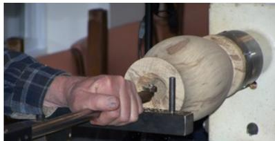
Do outside shape first, before working on hollowing out the inside, which allows you to see where the laser light is hitting.
