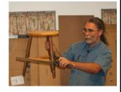
Leg fitting: Todd showed how the legs then fit into the seat. He uses flat board scraps tacked into a triangular support system to hold the legs in place to measure for the length of the stretchers' dowels. This system supports the splay, so you end up with equal distances between the legs.
