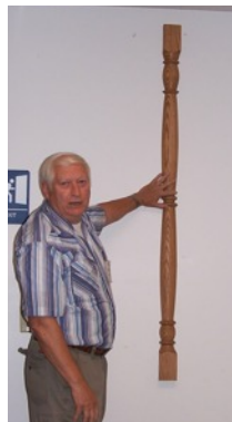
Barry Stump 6' 1/2 column room/wall separator Oak, Cut lengthwise, taped/glued together then turned. The halves were then reattached lengthwise
