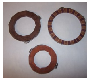
Examples of using circular clamps for segment gluing.
