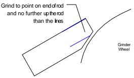
Rotate Rod so that next blue line is straight up. Grind next bevel.
