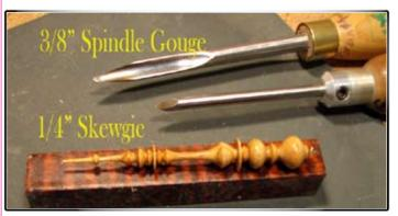
used to shape the finial. With opposing finger support, the skew chisel is used only for refining a straight line section. The tool rest is constantly moved closer to the piece being careful to first stop the lathe and ensure the piece clears the rest before turning back on. Note: A finial always looks thinner on the lathe (horizontal) so look down on it (vertical) to get a better picture of its actual size.
