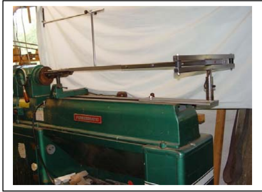
Hollow turning tool by Elmer Absher You can connect a vacuum hose to the end of the handle to suck up the shavings as you are turning.
