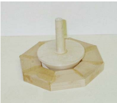
(Left) Jig for holding segmented turning blanks by Mike Galloway
