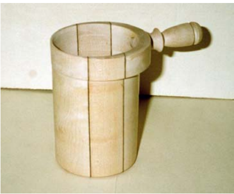
(Left) Eccentric-turned cup by David Smith. The thicker wall on the right permits fastening a handle while the thinner wall on the left reduces the weight.
