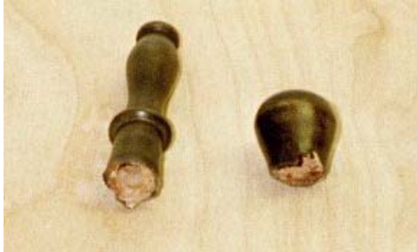
(Right) Glue chuck for holding small objects. Dale McCoy.
