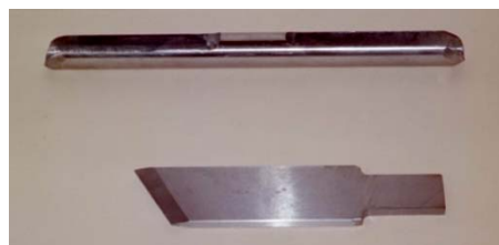
(Left) Selection of projects turned during hands-on session with Harry Memelink (Right) Homemade skew chisel and double-ended gouge by Elmer Absher
